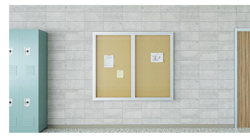
Large Contemporary bulletin board cabinets feature a heavy-gauge rectangular aluminum housing with satin anodize finish in 1-1/2" x 3" or 1-3/4" x 4"; inside depth of 3" cabinet is 1-3/4"; inside depth of 4" cabinet is 2-3/4". Tackable panels can be Claridge Cork, Fabricork, Guilford of Maine Fabric, or Hook-Fab.
